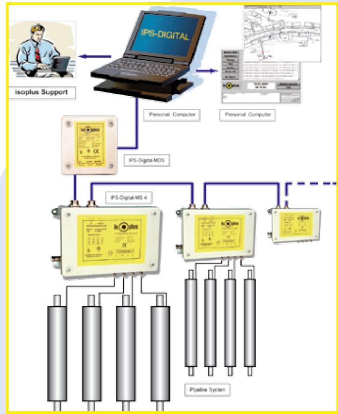
One single software will be sufficient for the control of the complete IPS-Digital-Network. All units of the **IPS-Digital-Hardware** are using this **IPS-Digital-System**-Software. The following basic logic functions will be carried out:
