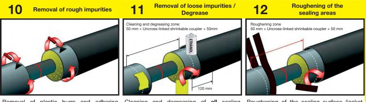
Removal of plastic burrs and adhering impurities on all sealing surfaces with a triangular scraper.
