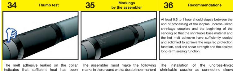
indicates that sufficient heat has been introduced. Additionally, through the thumb test, the collar is displaced axially to the beads which immediately recede back to a smooth surface when sufficiently warmed through.
