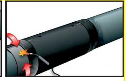
Start the shrinking process at the sealed end (12:00 clock position) and continue in the direction of jacket pipe.
