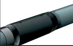
Only unpack the collar and remove the protective film immediately prior to processing (danger of contamination). Based on the centring marks, position the bevelled collar end and loosely wrap around the pipe. Remove the protective film from the second straight and overlapping end of the integrated sealing flap.
